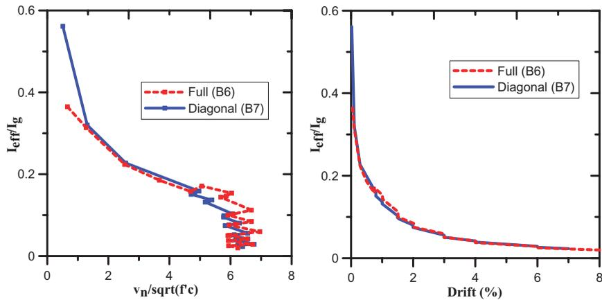
Figure 11. Effective stiffness versus (a) shear stress and (b) drift
