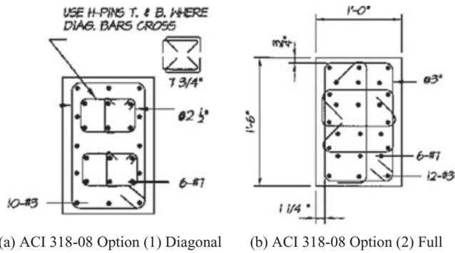
Figure 9. Link beam tests:  $l/h = 3.33$ , one-half scale
