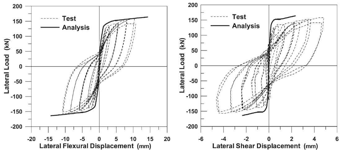
Figure 4. Load displacement relations: (a) flexure, (b) shear
