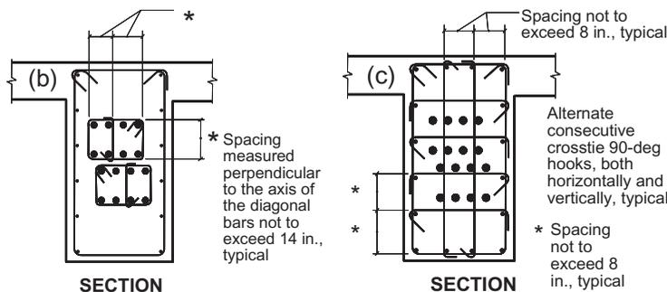
Figure 8. Link beam detailing (a) test, (b) ACI 318-05, (c) ACI 318-08 proposed
