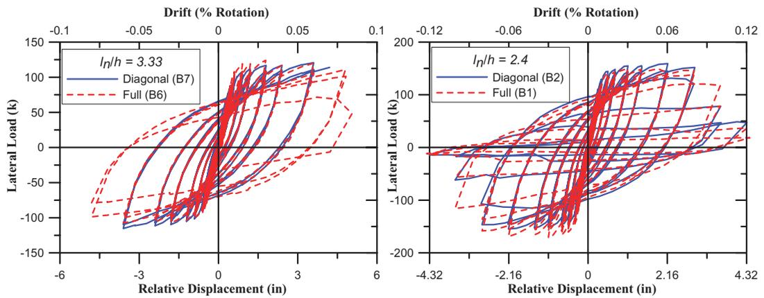
Figure 10. Load deformation relations
