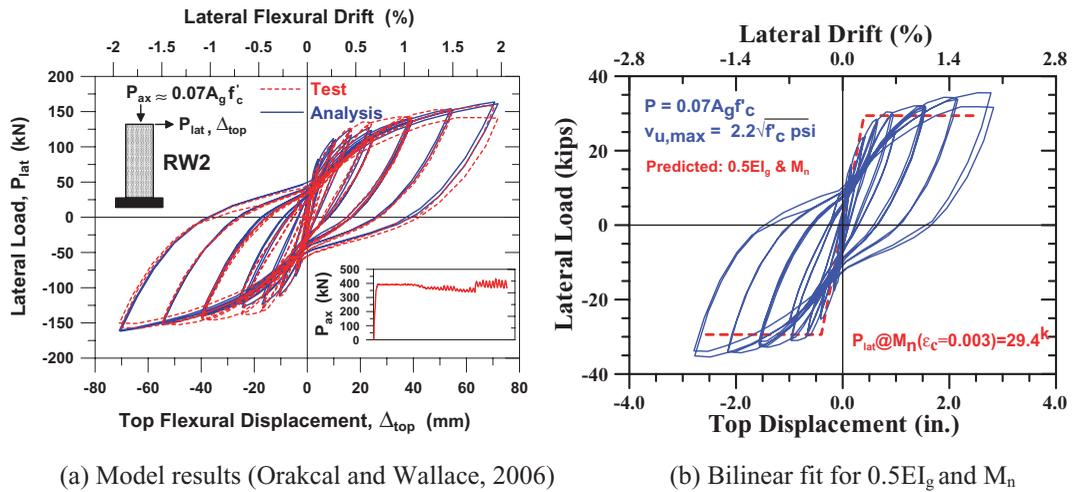
Figure 1. Test results for specimen RW2
