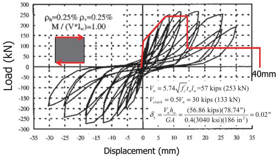
(a) Proposed shear backbone relation with test by Hidalgo et al. (2002) (strength degradation and residual strength defined by FEMA 356 (2000))
