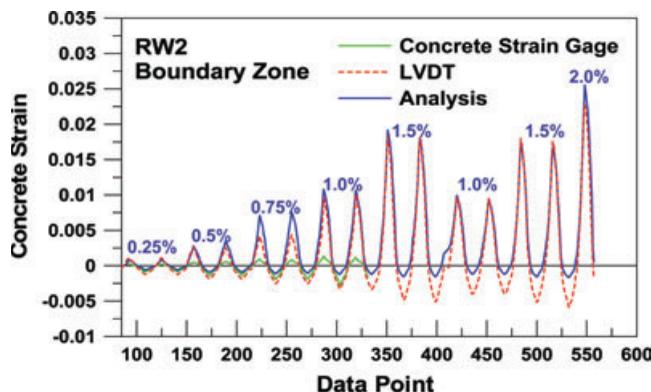
Figure 3. Wall average strain at critical section
