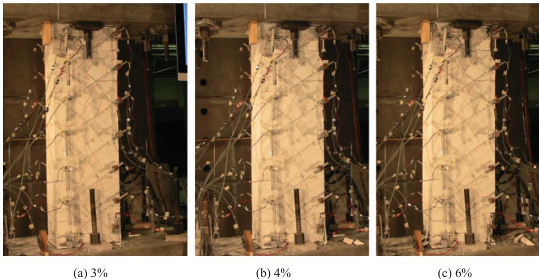
Figure 12. Damage photos of Beam #7:  $l/h = 3.33$  specimens
