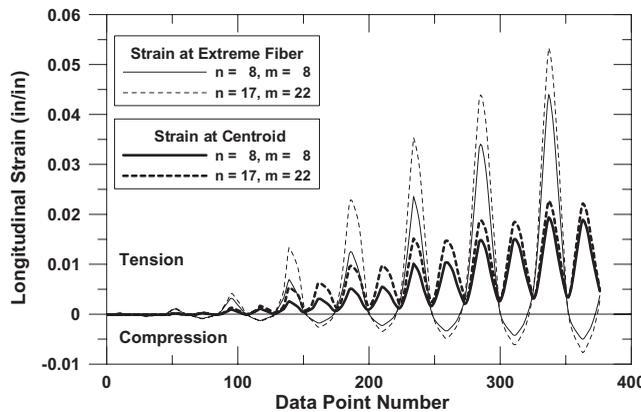
Figure 6. Wall critical strain sensitivity to model parameters
