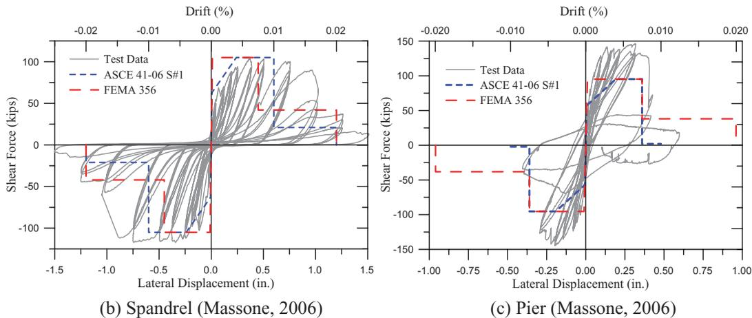
Figure 13. Wall segment force versus deformation relations
