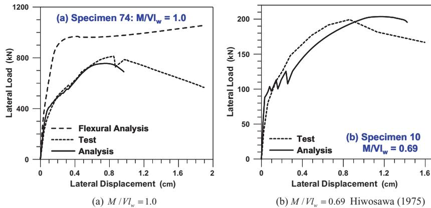
Figure 14. Coupled analysis: (a)  $M/Vl_w = 1.0$ , (b)  $M/Vl_w = 0.69$
