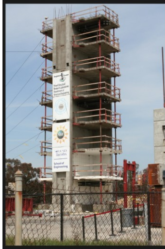
Figure 3: Photograph of the site showing the Seven-Story building built on the Shake Table.
