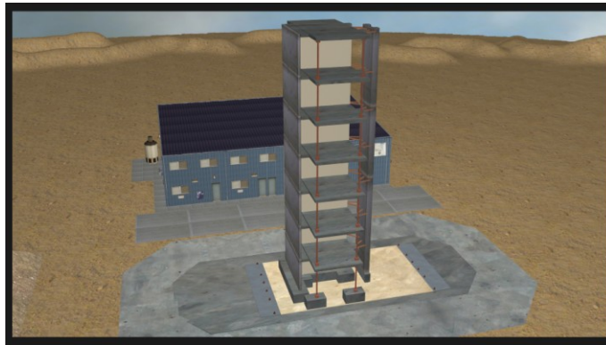
Figure 4: A 3D model of the experiment site. The seven-story building is built on the Shake Table. The machine room and monitoring facility is located in the rear building.
