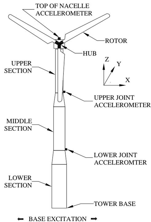
Figure 2: Accelerometer Locations
