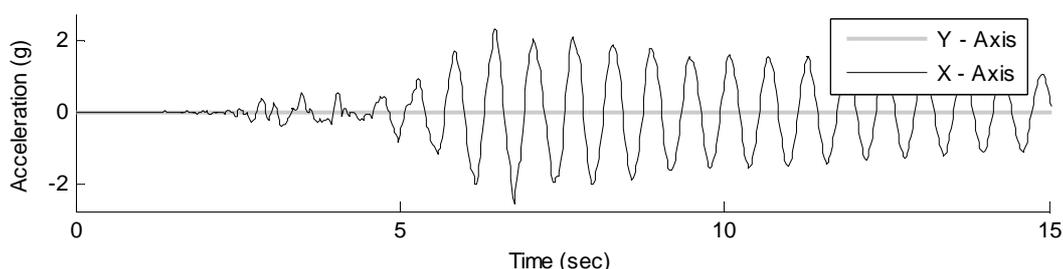
Figure 6: Acceleration Response at Top of Turbine for Strong Component Westmorland Earthquake Simulation
