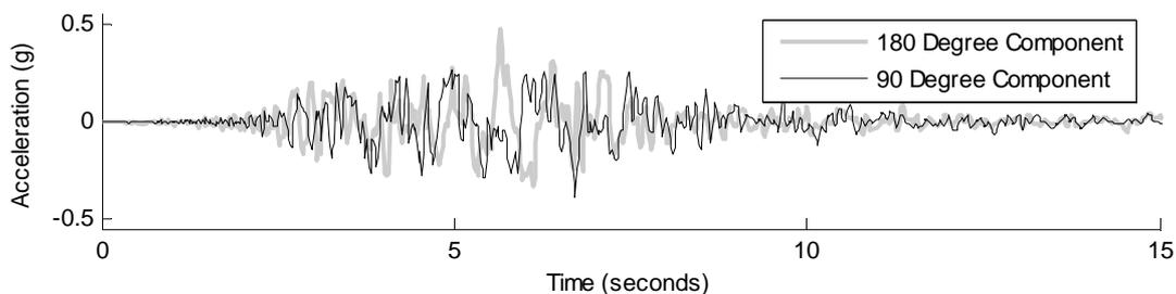
Figure 5: 1981 Westmorland Earthquake Acceleration Time History Recorded at Fire Station
