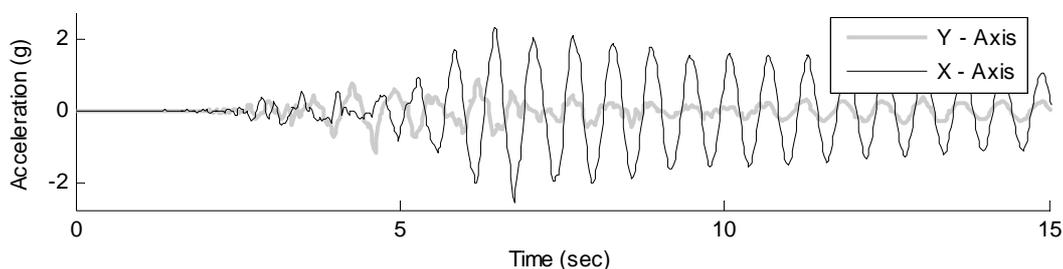
Figure 7: Acceleration Response at Top of Turbine for Bi-directional Westmorland Earthquake Simulation
