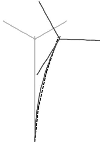
Figure 3: Observed (dashed) and Predicted (solid) 1<sup>st</sup> Mode Shape
