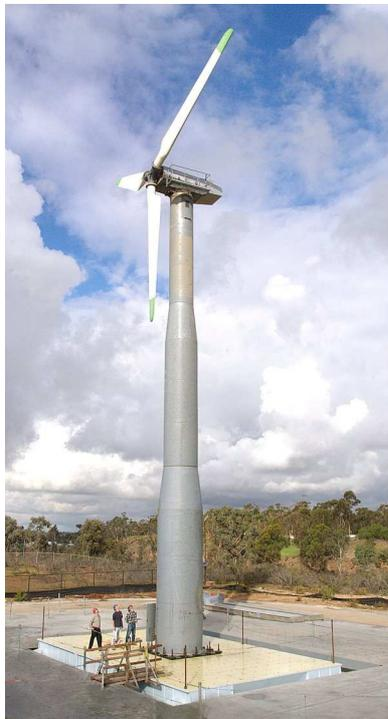
Figure 1: Shake Table Setup
