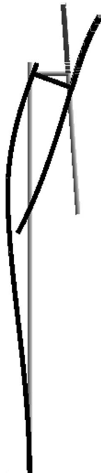
FIGURE 13 OpenSees Model II 2 nd longitudinal mode (9.7 Hz).
