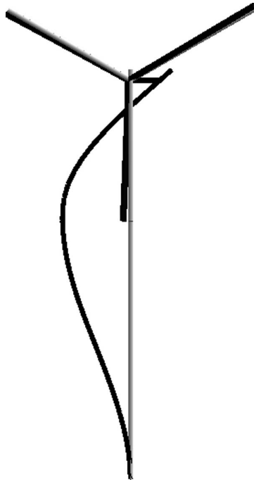
FIGURE 14 OpenSees Model II 2nd lateral mode (12.1 Hz).
