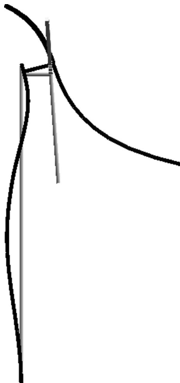
FIGURE 15 OpenSees Model II 3rd longitudinal mode (21.5 Hz).
