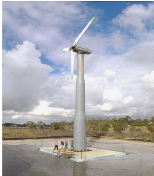
Figure 1. NEES-UCSD LHPOST with a full-scale 21 m high wind turbine mounted on it.
