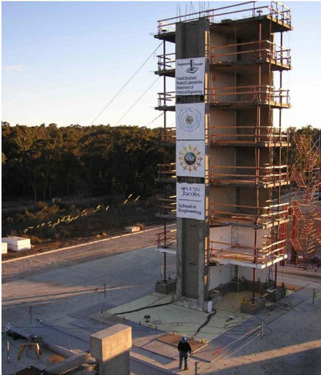
**Fig. 1.** Seven-story full-scale R/C building slice, 19.2 m high
